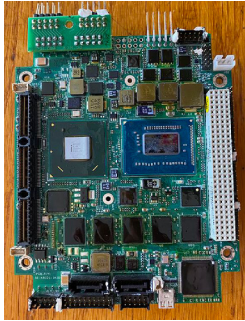
Single Board Computer in Lich Korsar made with Infineon Technologies MOSFETs
